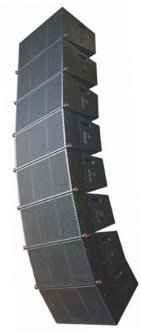
**The PLA21021** is a 2-way true line source enclosure, with a controlled dispersion pattern of 110 x 15, using advanced waveguides for the 2 x 1" Neodymium drivers, and soundguides for the two High-power neodymium 10" woofers, controlled dispersion is achieved over a very impressive frequency range.
