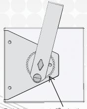
Each hole represents 50 using the quick-release springe for fast and accurate aiming.
