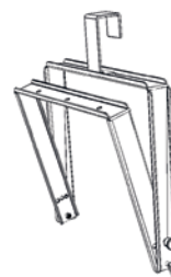
Cradle for installing with hook or clamp with adjustable tilt
