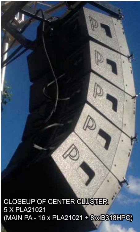
LIVE STAGE 16x PLA2821 - LINE ARRAY 8x SUB6HP - 2x18" SUBWOOFERS 6x CXL152MP - STAGE MONITORS
